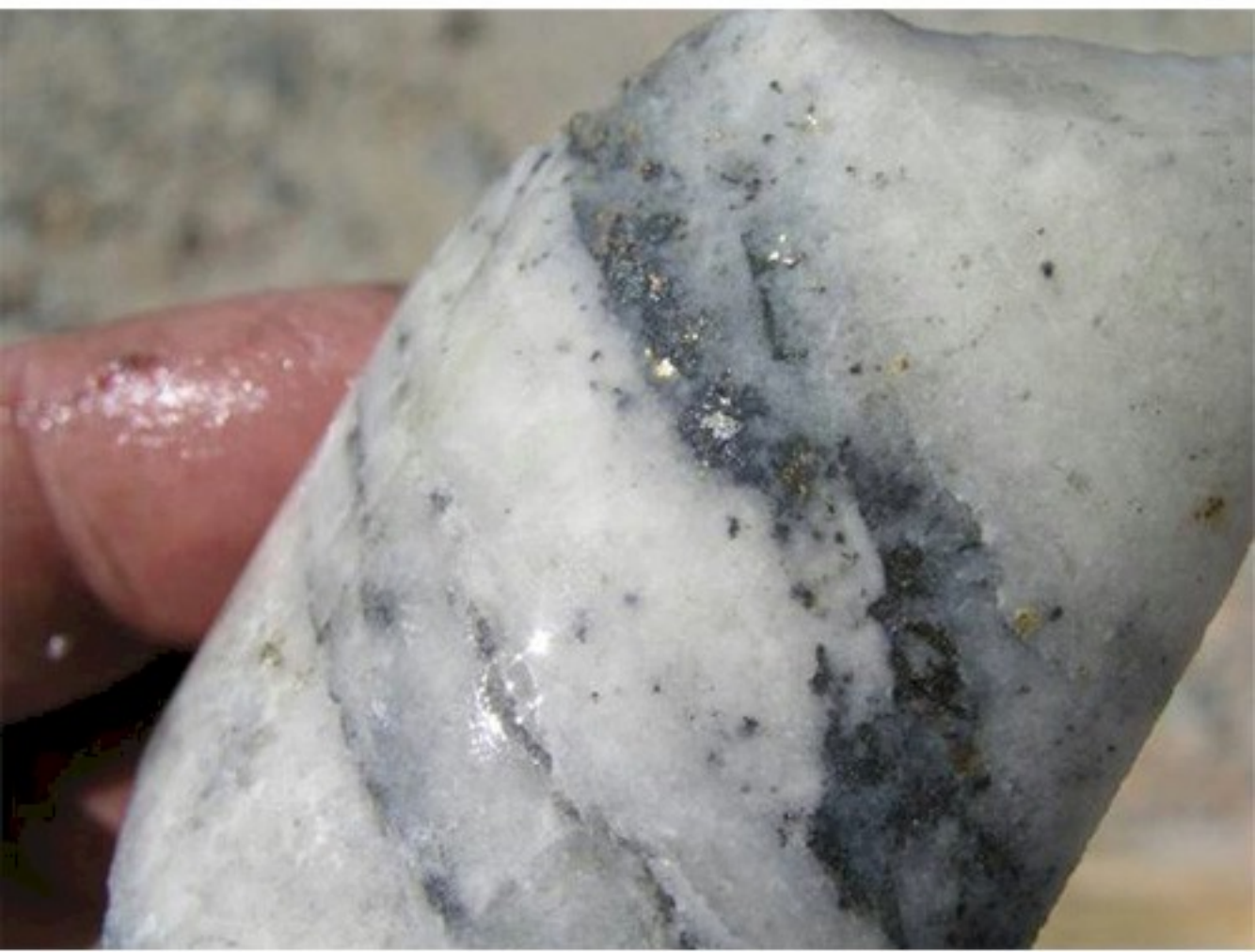
Drill core #12 219.06 g/tonne gold over 4.50m
