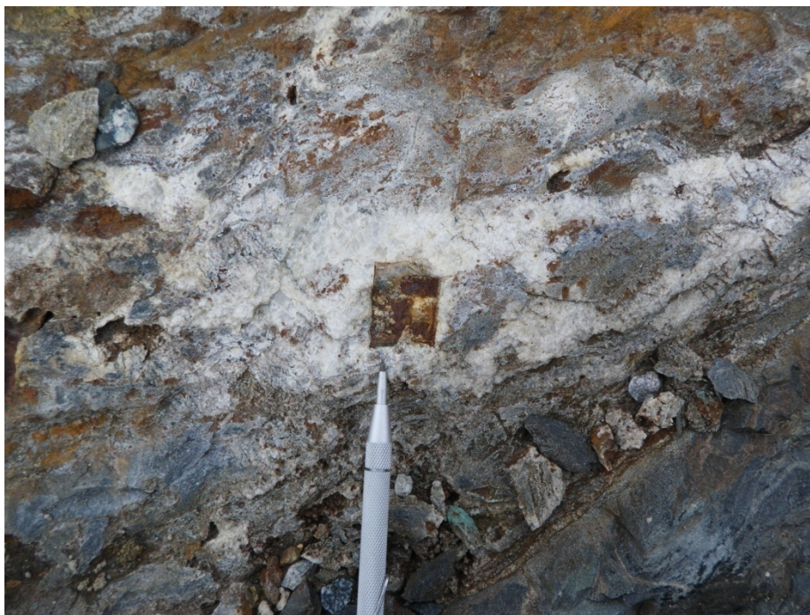
Figure 8: Oxidized Mineralization in the Main E-W Shear Zone. With Coarse to Fine Grained Pyrite Boxwork
