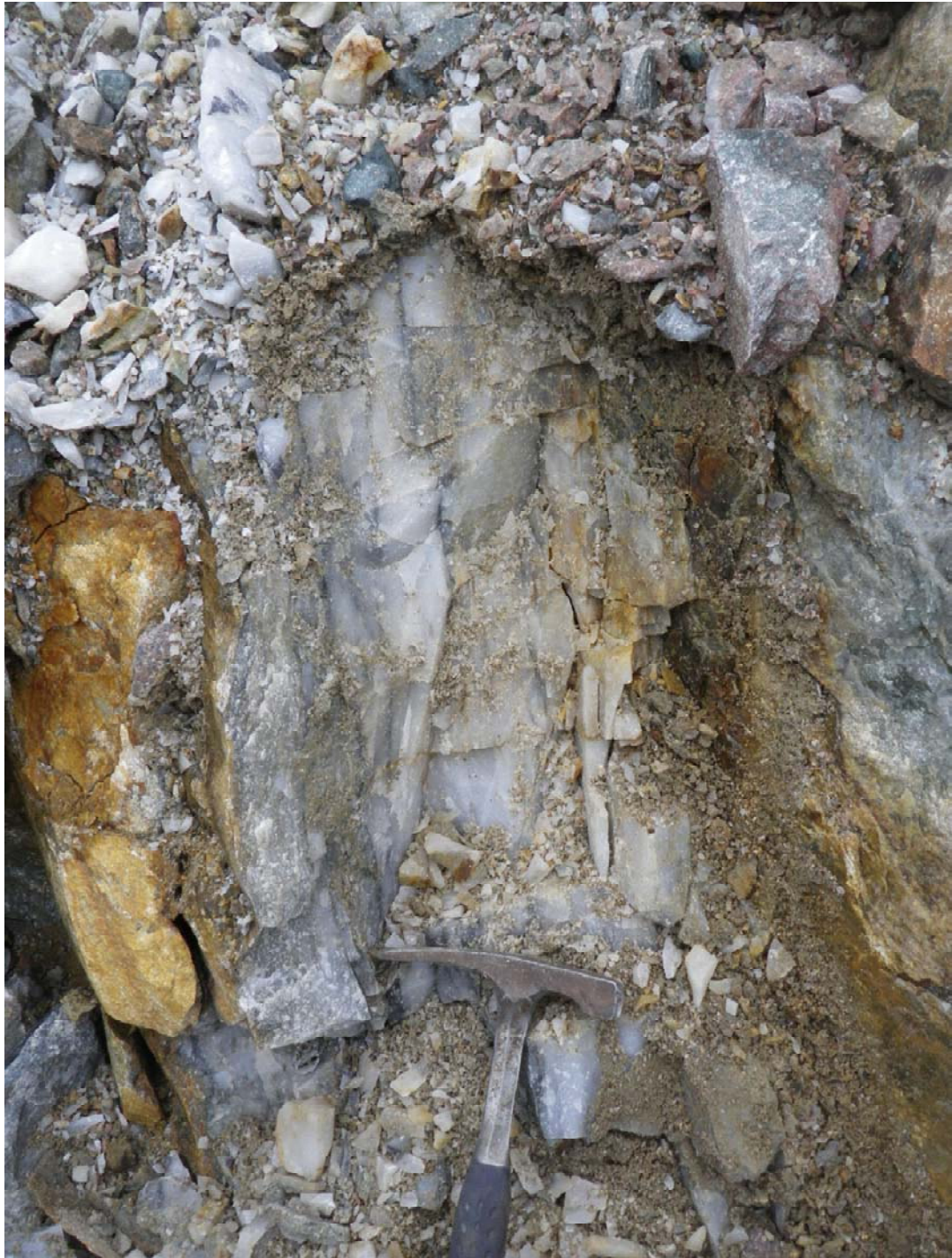
Figure 10: E-W Sub-Vertical Sheeted Quartz-Carbonate Vein with Fine-Grained Pyrite Stringers
